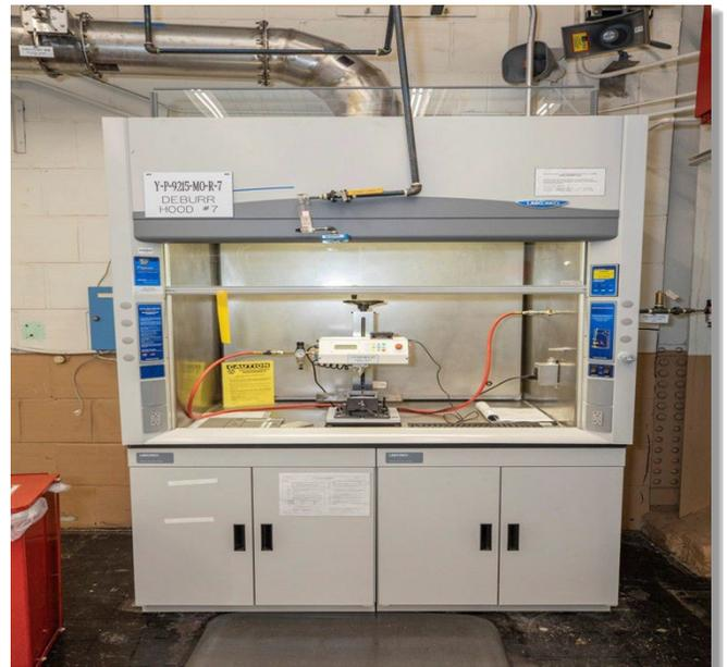
**Figure 15. Dot peen marking machine.**
